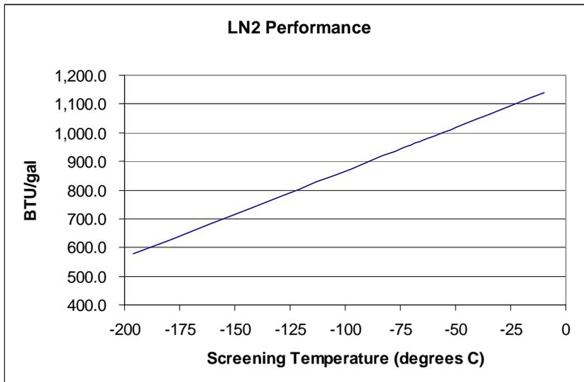
Figure 6 – LN2 Performance for various screening temperatures
