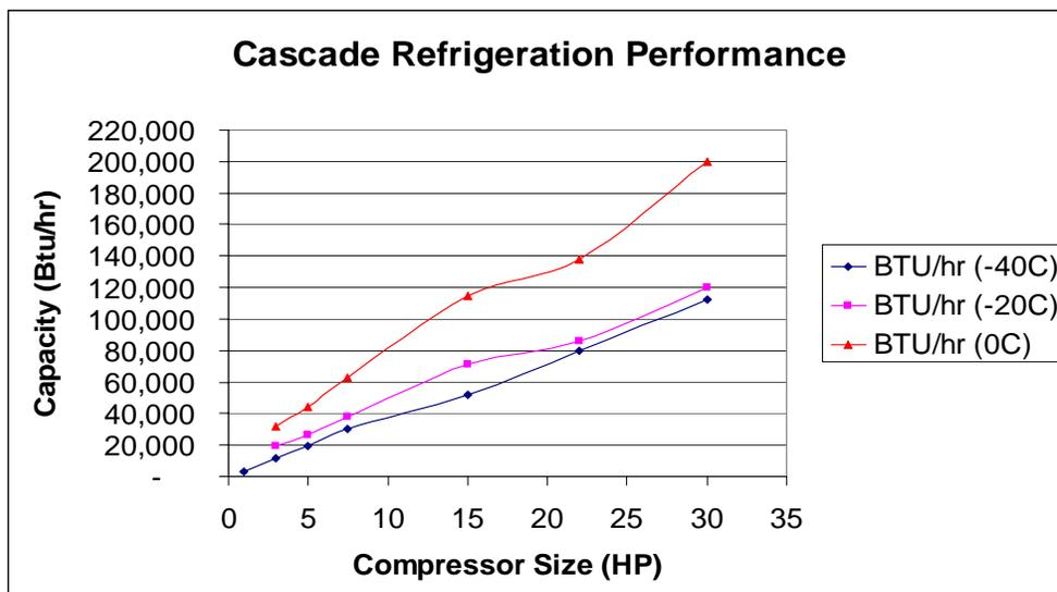
Figure 5 – Cascade Refrigeration Performance for various compressor sizes
