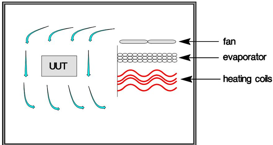
Figure 3 – Single zone chamber layout
