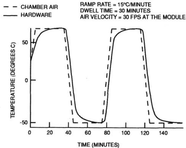
Figure 2 – Product response for the proper airflow case
