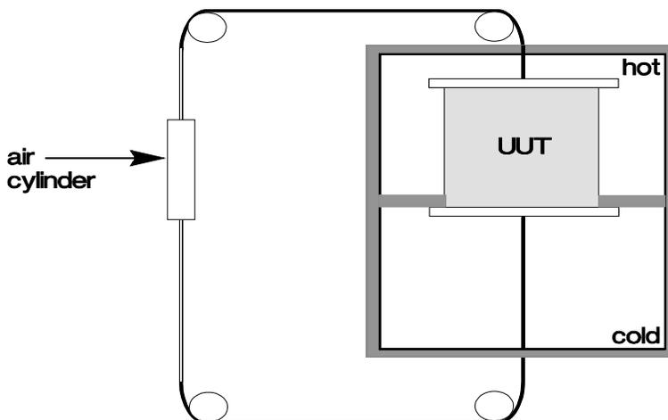
Figure 4 – Two zone air-to-air chamber
